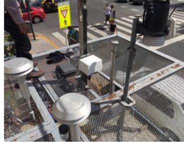
Fig. 3 PRAXIS monitor installed on the EPA Reference Air Quality Monitoring Station - APRa Córdoba
